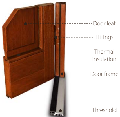
Cross-section of standard door
